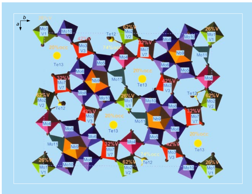
Figure 4.8 Schematic representation of the structure (projected along [001]) of the M1 complex oxide phase of the oxidation catalyst composed of Mo–V–Nb–Te–O (red: \text{Mo}^{6+}/\text{V}^{5+} ; green: \text{Mo}^{5+}/\text{V}^{4+} ; purple: \text{Mo}^{6+} ; orange: \text{Nb}^{5+} ; teal: \text{Mo}^{5+} ; pink: \text{Mo}^{6+}/\text{Mo}^{5+} ; yellow: \text{Te}^{4+} ). 20
